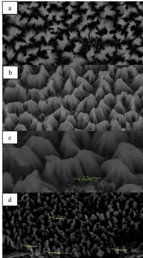
**Figure 3.** Result of MACE after 45 minutes. (a) showing a SEM image in plan view (b) at 30°-point view, showing the formed and positioned nano-pillars (c) showed a growth profile of Si nano-pillar and (d) showed a uniform separation of nano-pillars.
