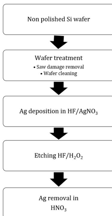
**Figure 1.** The process flow involves in two-step MACE process
