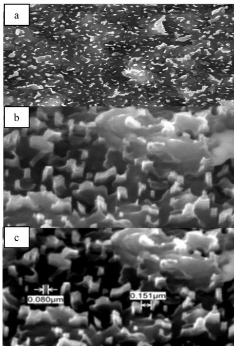
**Figure 2.** Result of deposition of Ag particles where (a) display a white spot all over the Si surface (b) presence the porosity of a Si wafer and (c) display a sample is separated and etched after being deposited in Ag/NO<sub>3</sub> after 4 minutes.
